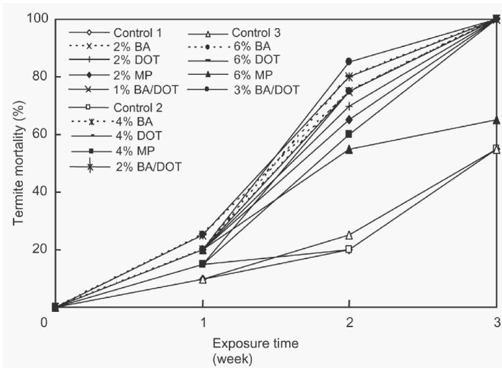
Figure 7. — Termite mortality after 3-week termite test.
