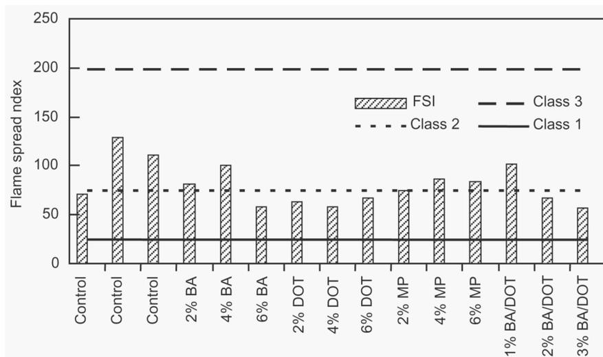
Figure 4. — Flame spread index for OSB specimens.
