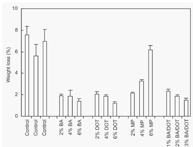
Figure 8. — Weight loss during termite assay.
