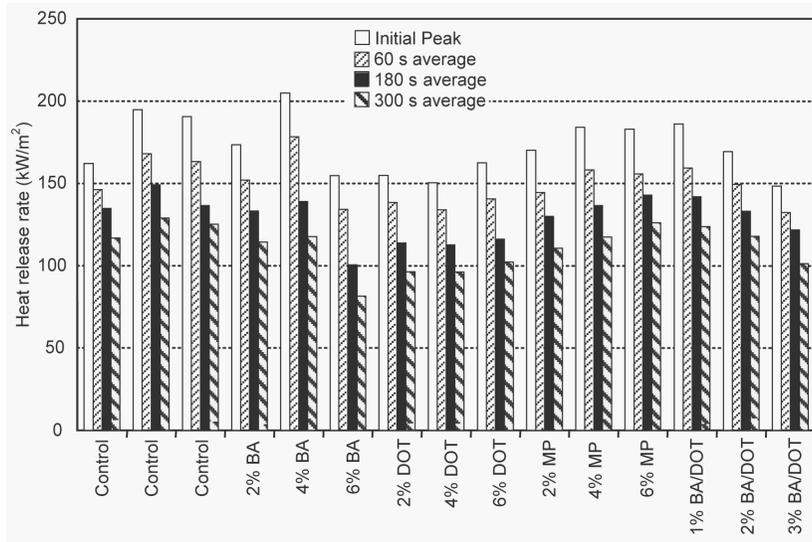
Figure 2. — Heat release rate (HRR) of OSB specimens.
