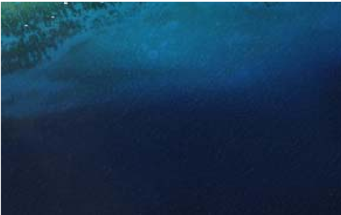
Figure 5. Image of Looe Key before sea surface correction was applied showing ripples on the sea surface.
