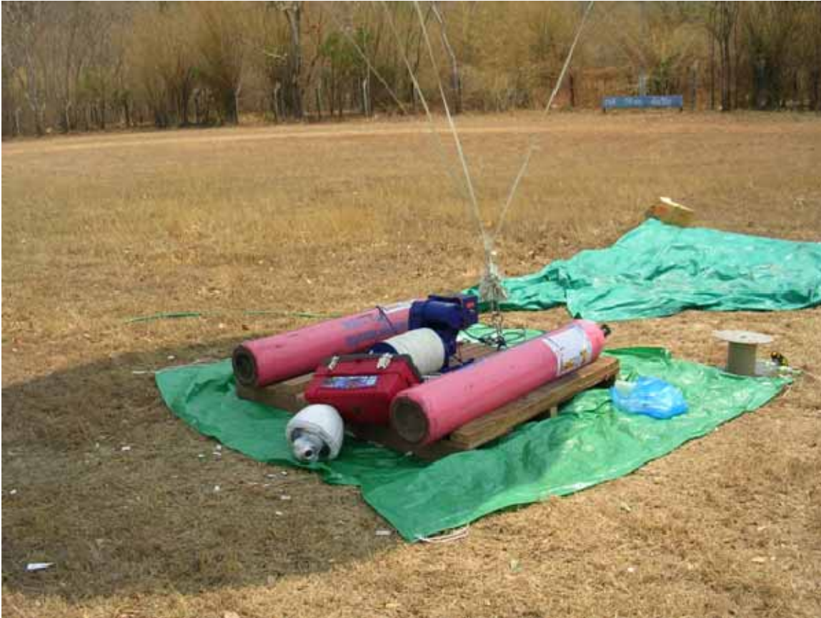
Figure 7. Balloon Platform with Winch and Helium Bottles
