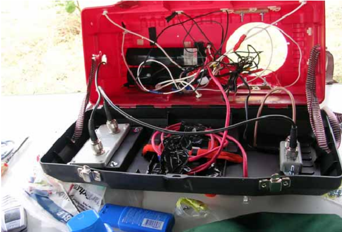
Figure 10. Tool Box Payload with 2W Amplifier and Camera Mount
