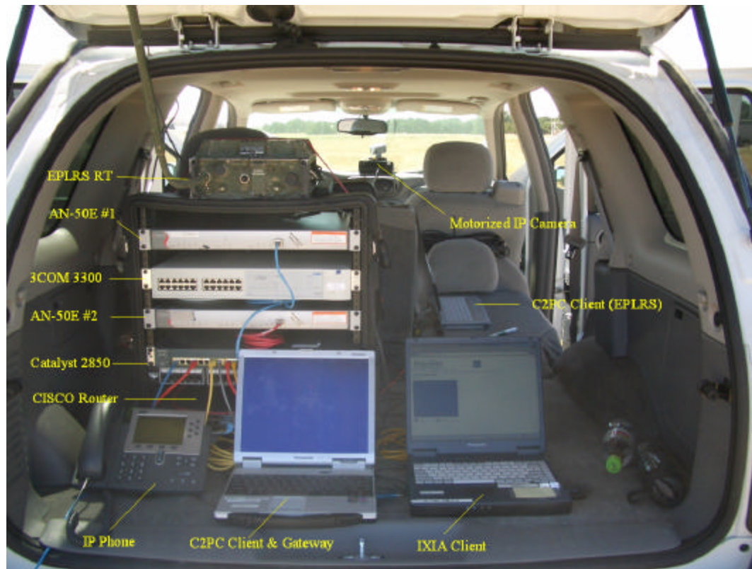
Figure 33. LRV Communications Package for Mesh Bridging
