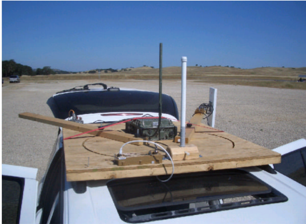
Figure 34. EPLRS RT Relocated Mounting for ATDNG Experimentation
