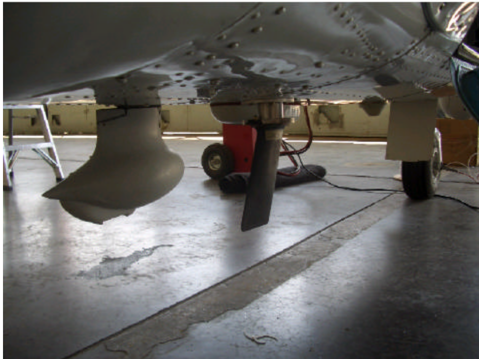
Figure 27. EPLRS UHF Blade Antenna Mount on Pelican (UAV Surrogate)
