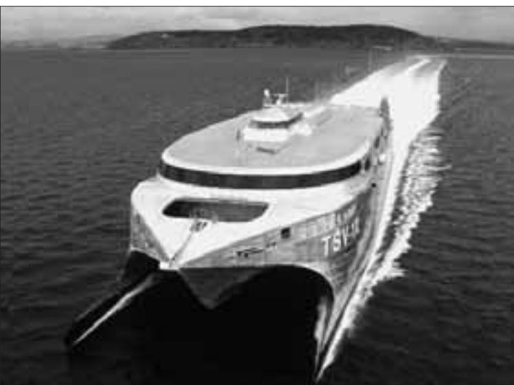
United States Army Vessel (USAV) Theatre Support Vessel (TSV-1X) Spearhead. The 98-meter USAV, with an average speed of 40+ knots, will transport troops and cargo. U.S. Navy photograph by Photographer's Mate 1st Class Brien Aho
