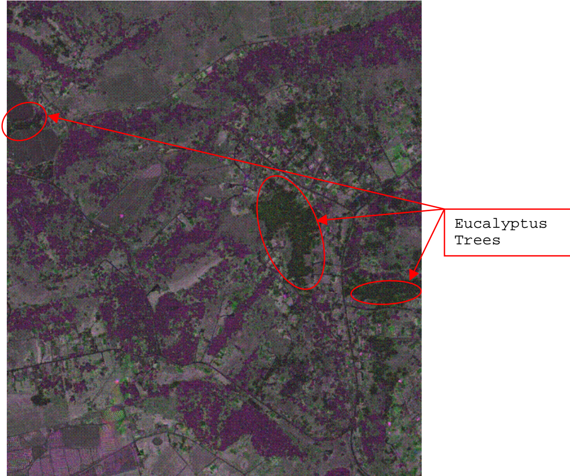
Figure 30. Image of Intensity Values Recorded from LIDAR Returns. Band 1 is mapped to Red, Band 2 is Mapped to Green, and Band 3 is Mapped to Blue
