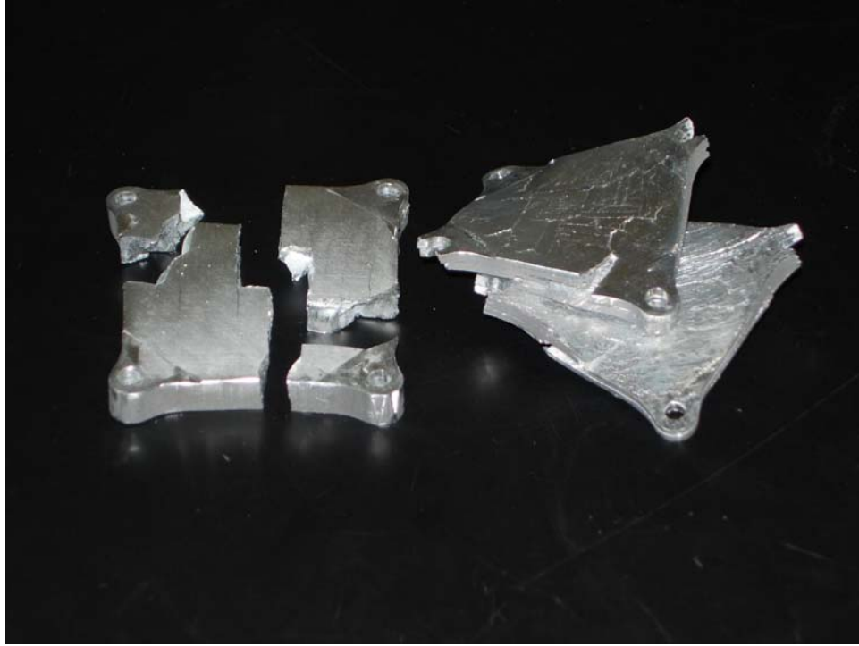
Figure 4-5. Anticlastic test specimens (FSP-left, AR-right) illustrating change in fracture mode.
