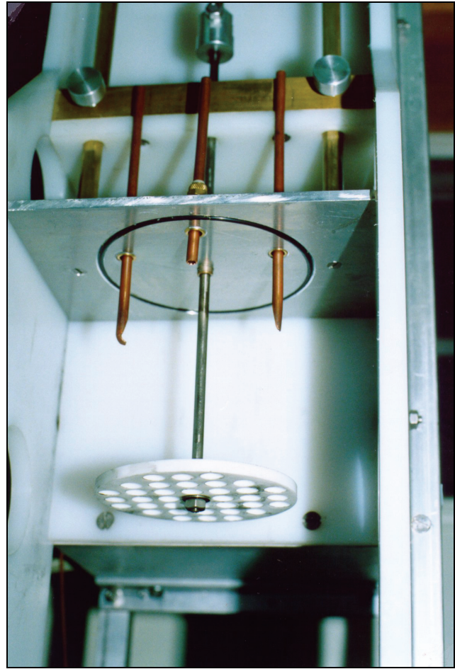
Figure 5. Perforated disk (grid) and suspension withdrawal tubes of PES
