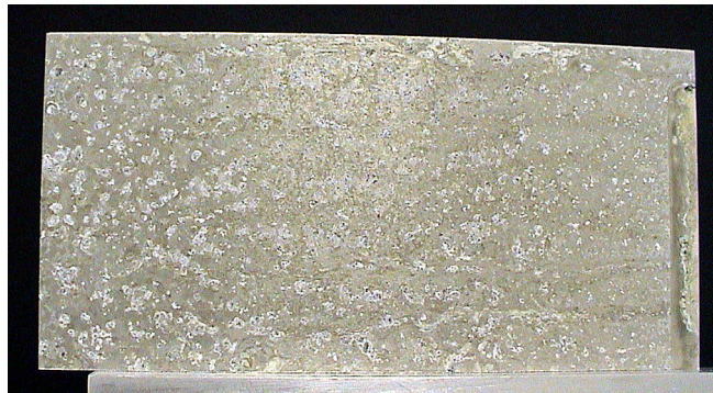
Figure 90a Visible image of corroded sample C1
