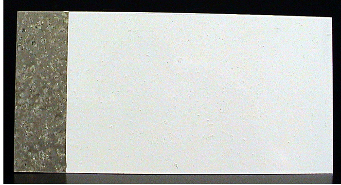
Figure 90b Visible image of the corroded sample C1 with 2.5 mil Gloss White
