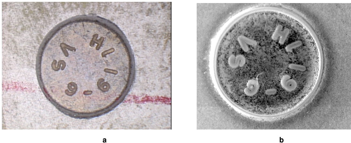
Figure 59 A visible image (a) of an unpainted fastener head, an IR image (b) of the same fastener covered with 3 mils of primer and topcoat.
