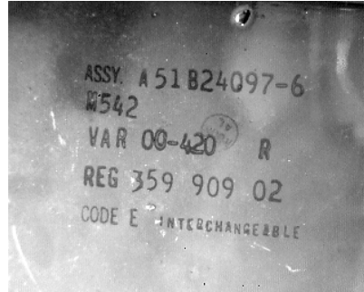
Painted Over Markings
