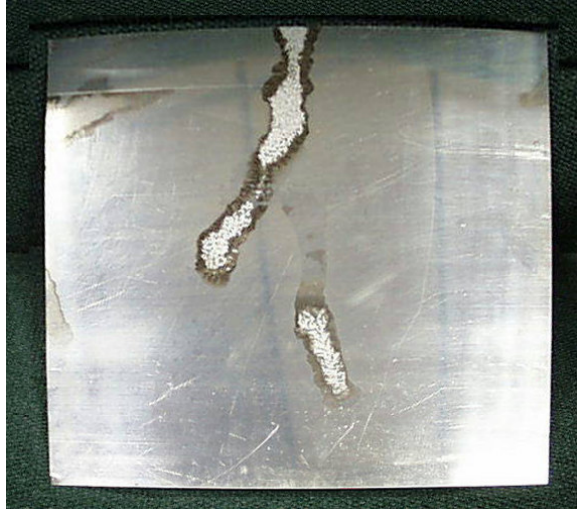
Figure 4 Photograph of a naturally corroded 12-in. x12-in. 2024 clad aluminum panel.
