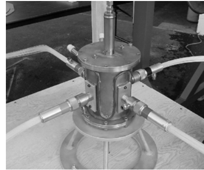
Figure 7. The solar receiver housing with four fiber cables connected.
