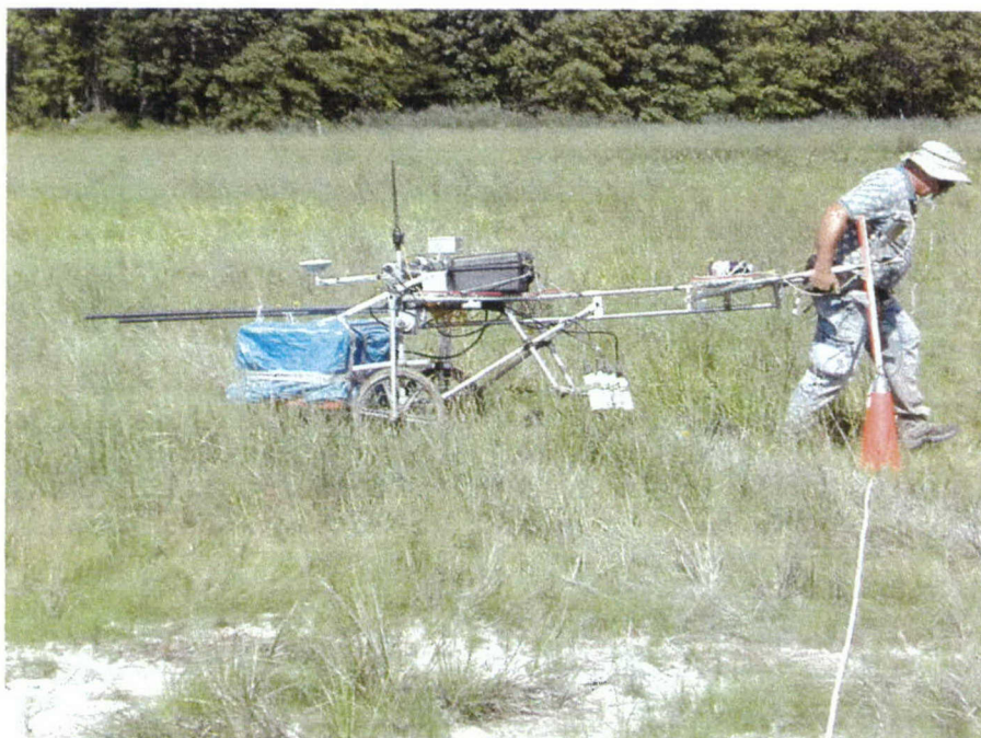
Figure 1. Demonstrator's system, simultaneous magnetometry and pulsed EM/man-portable.
