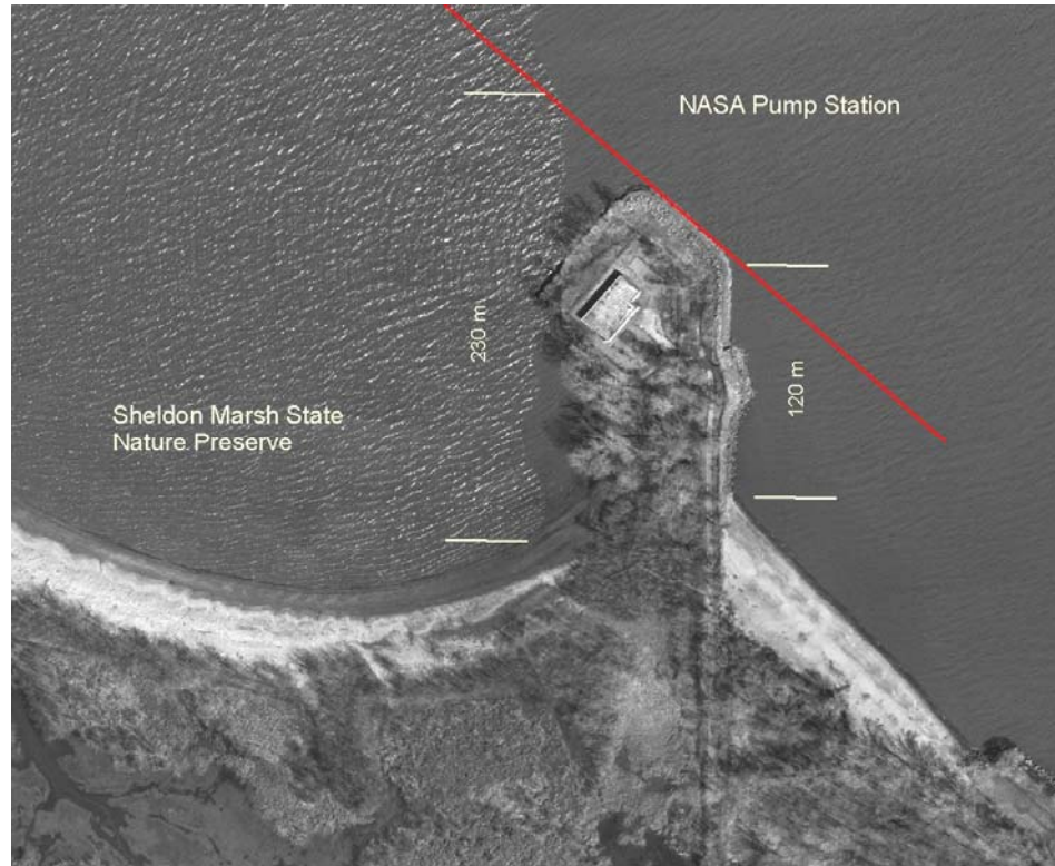
Figure 3. NASA pump station and beach at Sheldon Marsh, 12 April 2003 (north is to the top). The fact that beach has retreated on both east (updrift) and west (downdrift) sides indicate how little sediment is available in this system. Red line marks 1937 shoreline position (photograph courtesy of Erie County Auditor's Office)
