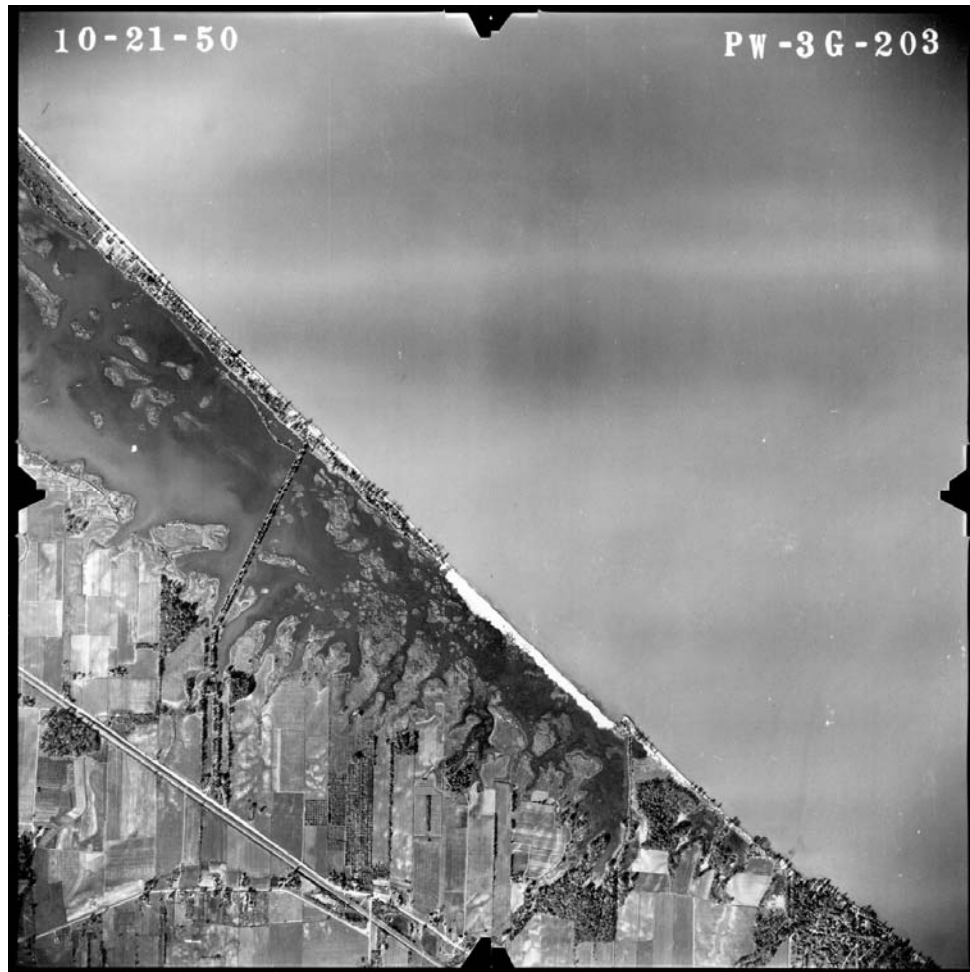
Figure 15. Sheldon Marsh, 21 October 1950. Ten years after pump's construction, beach had already retreated and lost most of its tree cover, to be replaced by washover fans (photograph courtesy of U.S. Army Corps of Engineers' Beach Erosion Board archives)
