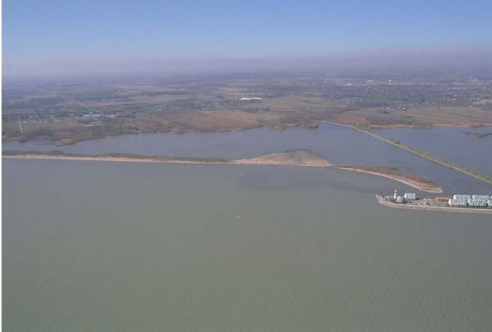
Figure 4. View looking south of west half of Sheldon Marsh, 13 April 1999. Armored spit on right is now easternmost end of Cedar Point Peninsula, but at one time, beach was continuous (photograph courtesy of U.S. Army Engineer District, Buffalo)
