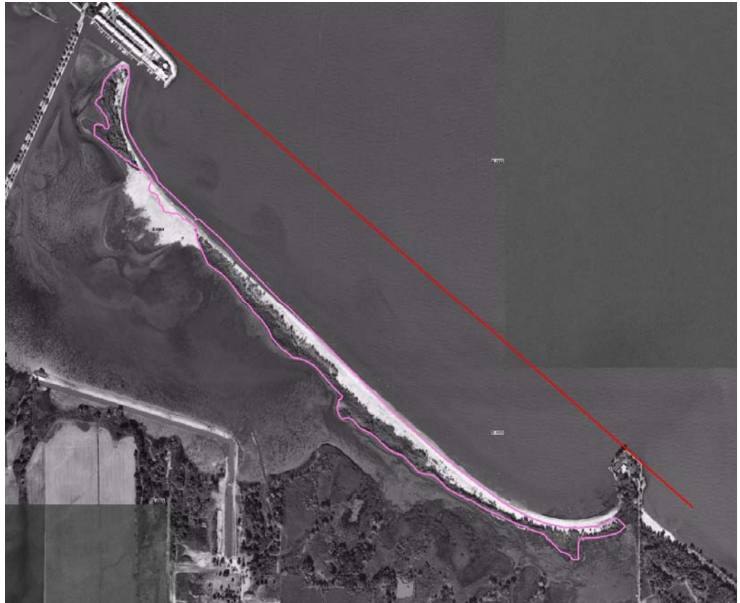
Figure 23. Sheldon Marsh, 10 Oct 2000. Overall position of beach is little changed compared to 1997 (purple outline). Washover occurred between two narrow portions of 1997 beach (north is top). (Digital photographs from U.S. Geological Survey, downloaded from TerraServer USA Web site ( http://terraserver-usa.com/default.aspx ), projected in ArcGIS software)
