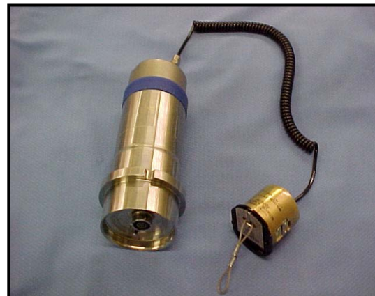
Hard Target Smart Fuze FMU-159 /B “Smart” Void, Layer, Time...
