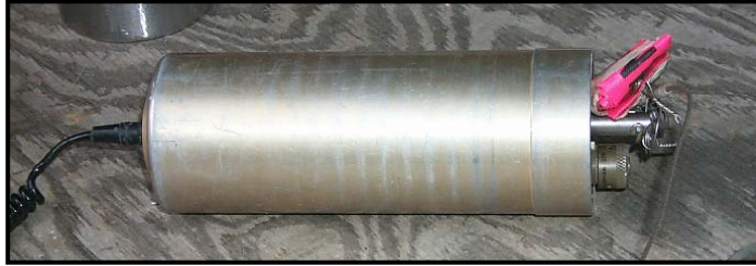
Electronic Bomb Fuze FMU-143 B/B Fixed Pyrotechnic Delay
