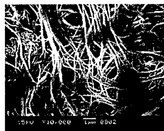
Fig.2 SEM of UHMWPE/CNTs composite fiber
