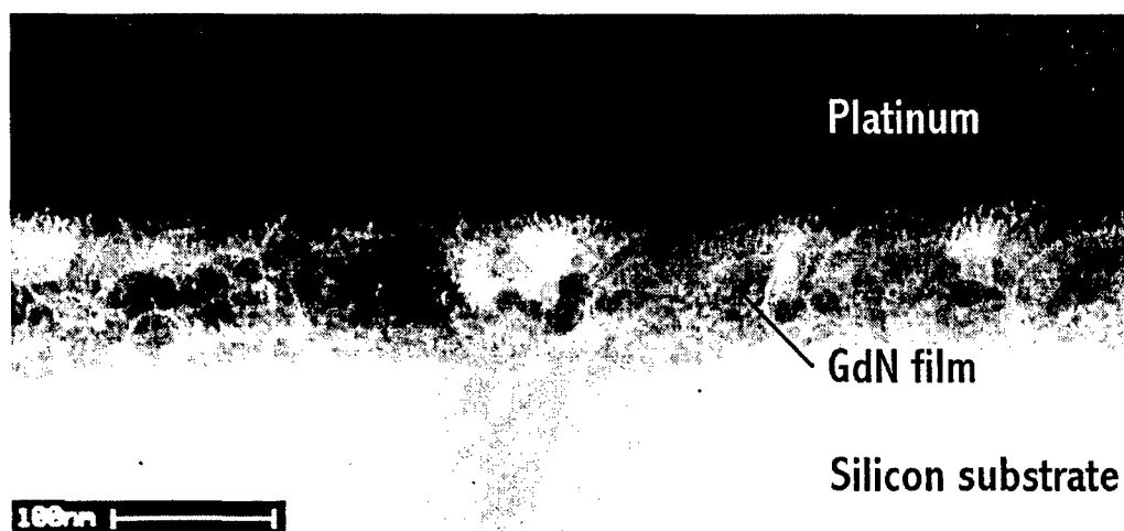
TEM image of the GdN thin film grown on a silicon substrate.
