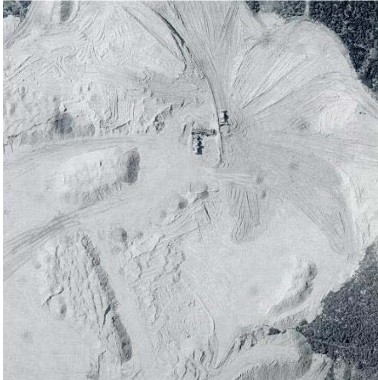
Figure D-6: NIIRS Level 6 Image. Clearly, the quality of this NIIRS 6 picture has improved over the NIIRS 2 example. Types of automobiles can be distinguished and trails can be discerned.
