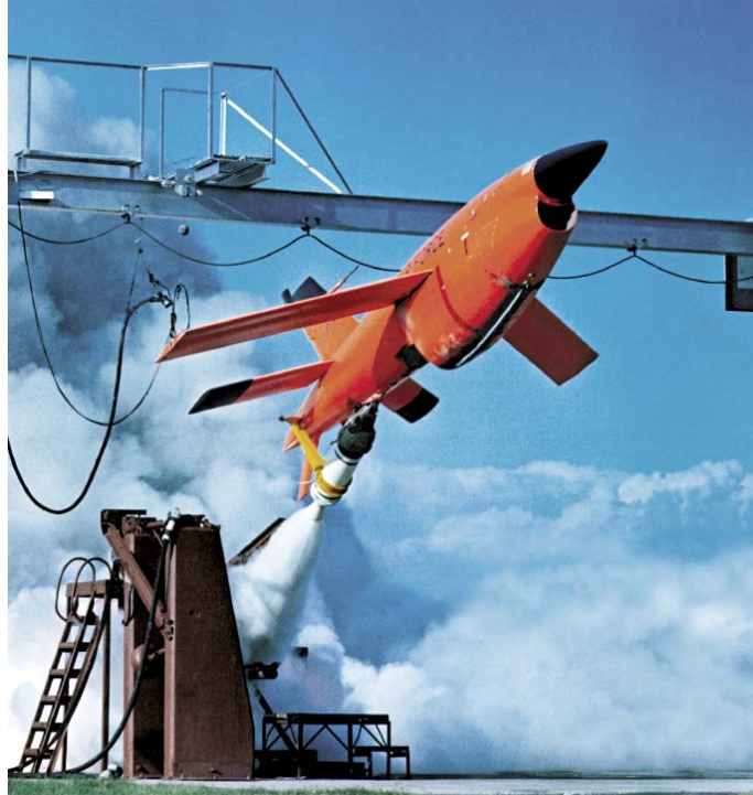
Figure B-3: Ryan BQM-34 Firebee (Northrop Grumman). This is the most successful and effective UAV program ever. Developed as a joint Army, Navy, and Air Force project in 1948, the UAV was initially designed to be a target vehicle and is now used in strategic and tactical reconnaissance roles.
