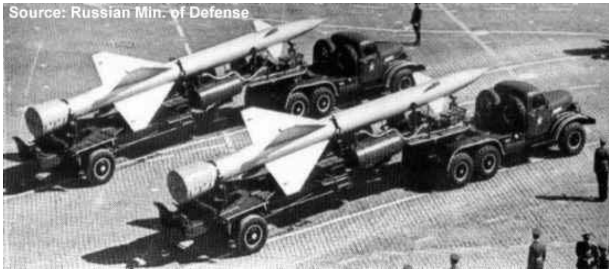
Figure A-2: SA-1 "Guild." The world's second operational SAM was the Russian SA-1 "Guild," which entered service in 1954. Intended to shoot down high-flying nuclear-armed bombers, it was a great achievement for its time. It was a fixed-site SAM that was deployed in two concentric rings around Moscow.
