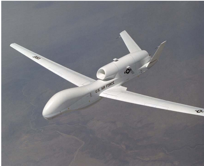
Figure B-4: RQ-4A Global Hawk (C.W. Controls, Inc.). The Global Hawk, built by Northrop Grumman, is a high-altitude (50,000-60,000 feet), long-range (15,535 miles max), and long-endurance (36 hours) UAV with a 116-foot wingspan, an allowable payload of 2,000 lbs, and a cruise speed of 343 knots. It has been used very effectively in recent military operations.
