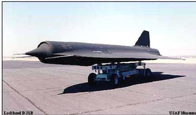
Figure B-2: Lockheed D-21 UAV (USAF Museum). The D-21 was a supersonic, air-launched UAV intended to capture images of areas that were unreachable by the SR-71, a fast, high-flying, long-range, stealthy manned reconnaissance aircraft.
