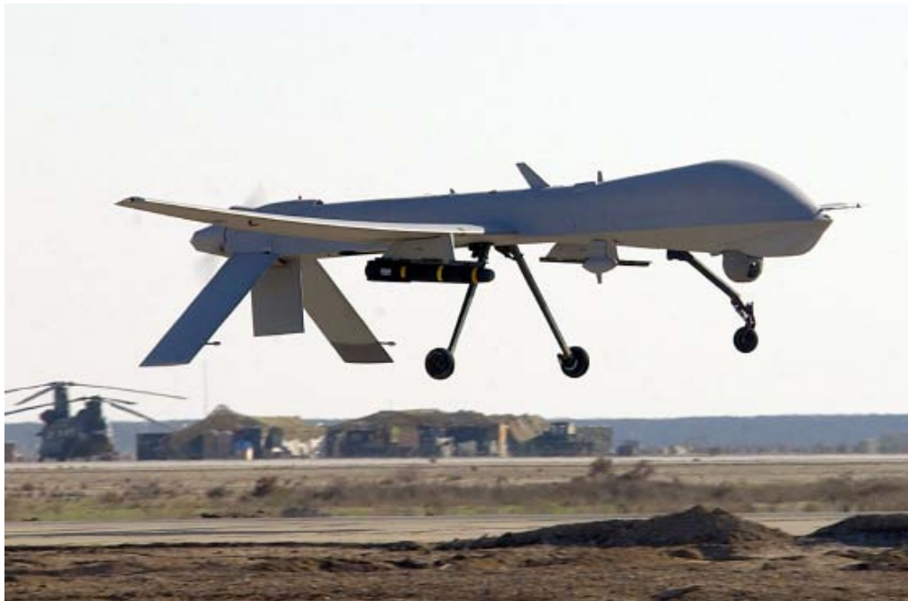
Figure B-5: GA RQ-1A Predator (Edwards AFB). The Predator is a short-range (2,302 miles), long-endurance (40 hours), and low-flying UAV with a loiter speed of 117 knots. It is unique in being the only operational UCAV within the US military.
