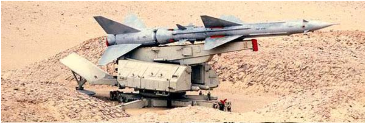
Figure A-3: SA-2 Guideline. The SA-2 is a long-range, high-altitude, two-stage missile still in use in many countries. It measures over 35 ft in length and travels at speeds in excess of Mach 3.5. It is famous for having been used to shoot down a U.S. U-2 spy plane flown by Francis Gary Powers in 1960.
