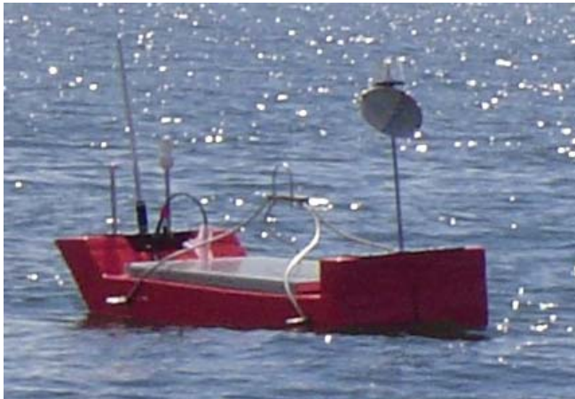
Figure 3. Racom gateway buoy. The racom buoy maintains a hard-wire connection to a repeater node attached to its mooring line. It provides a radio link between the undersea environment and the Seaweb operator on a surface vessel.
