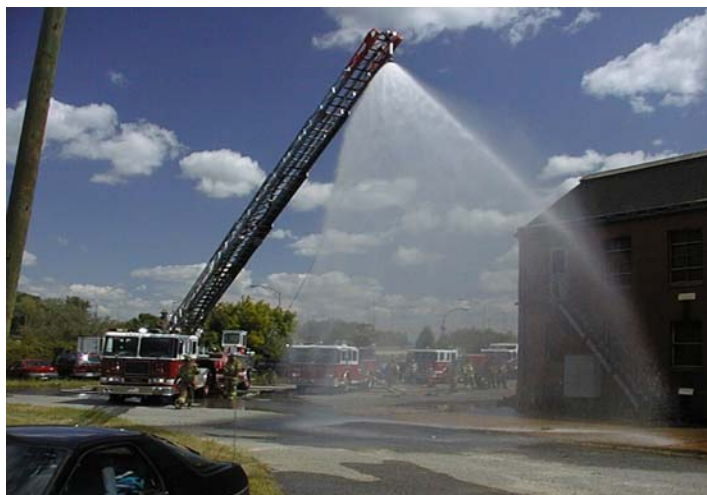
Figure 4-3. The Ladder Pipe Decontamination System (LDS)
