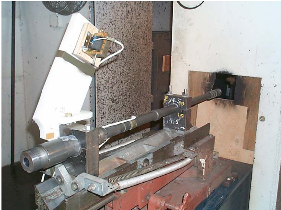
Figure 4. The 14.5-mm gun system.
