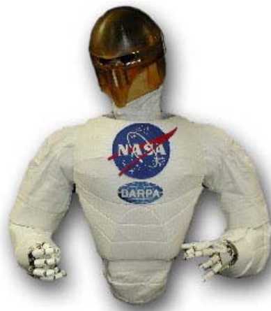
Fig. 1. Robonaut – NASA's Humanoid Robot
