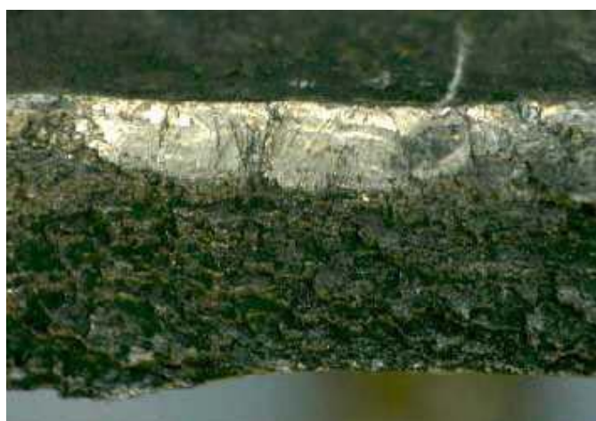
Figure 6: Fatigue crack in "overload" zone.
