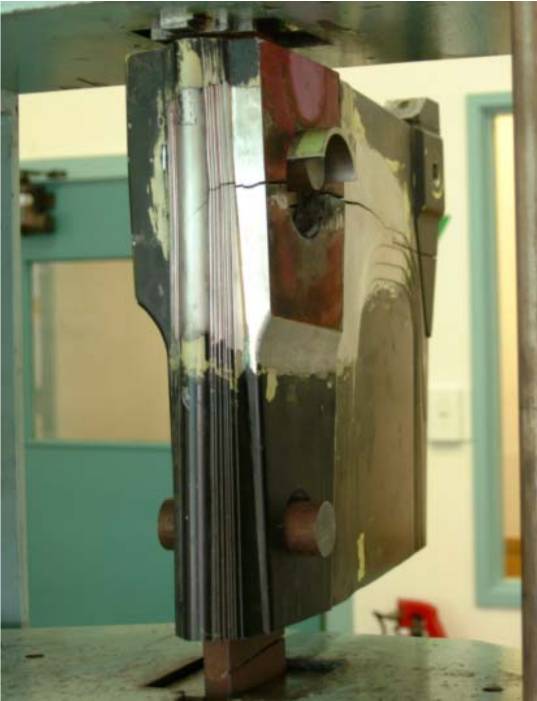
Figure 4. Application of a tensile load to simulate the crack opening displacement indicated by witness marks on the doubler. The aircraft was likely to have been flying with the crack in this configuration.
