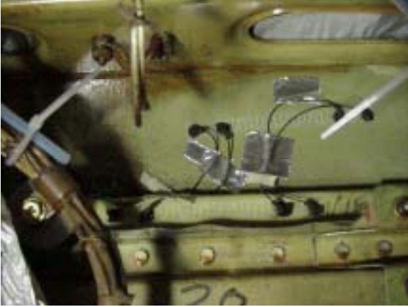
Figure 5. Surface sensors installed in the tail cone of a commercial DC-9 aircraft.
