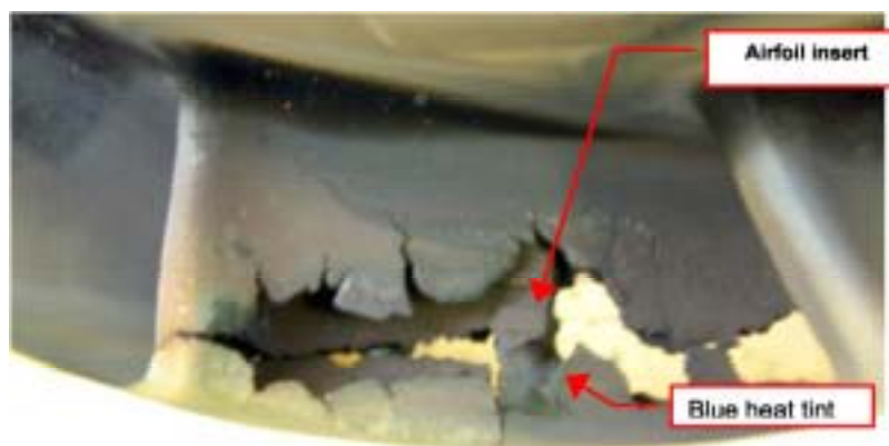
Figure 5. Photograph of the leading side of the perforated airfoil of CT vane 10 (Circled area in Figure 2). Note the rounded edges and the jagged cracking. Heat tinting of the surface is also observed (labelled).
