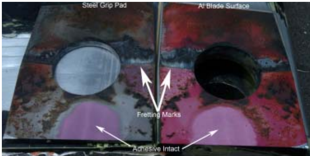
Figure 3. Adhesive surfaces after removal of the grip pad (left). The fretting marks indicate the crack opening displacement experienced in flight.
