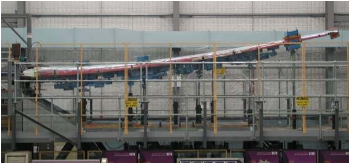
1: F-WELD Test Article Undergoing Cold Proof Load Test
