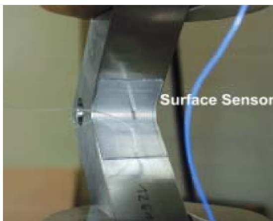
Figure 3. Surface sensor on a concave curve test coupon (from 1.)
