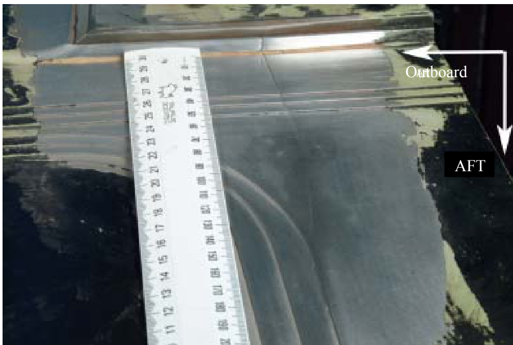
Figure 2. View of the crack propagating beyond the doubler.
