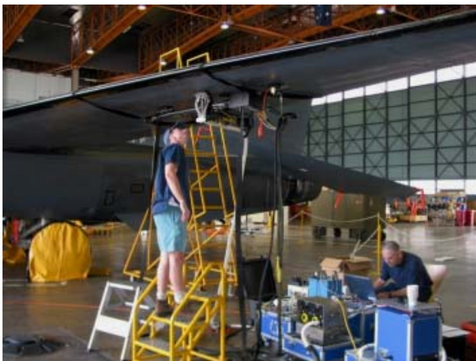
Figure 2 Automated ultrasonic inspection of Taper-Lok fastener holes in an F-111C wing using the SAIC Ultraspect-MP system.
