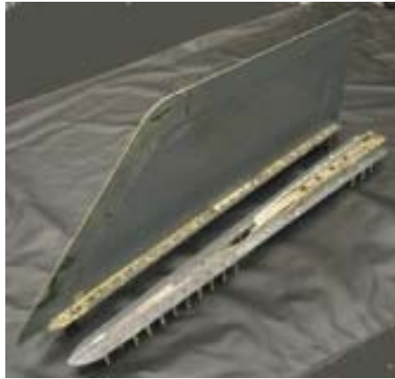
Figure 2: Failed strake next to a good one.
