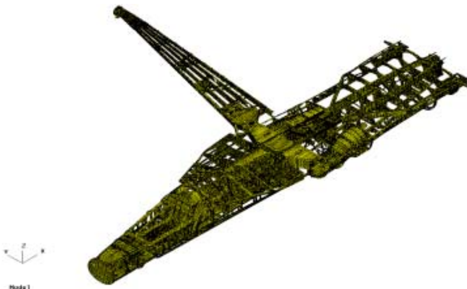
Figure 1: Major structural components of F-111 Internal Loads Model.
