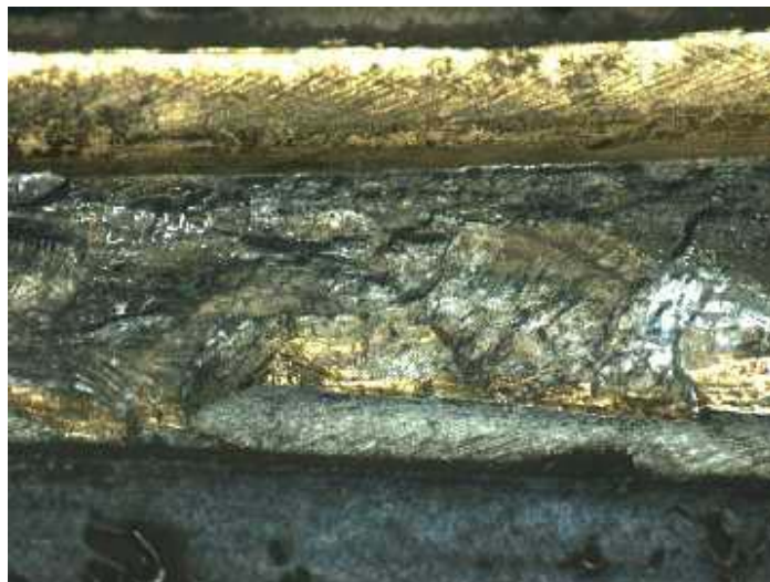
Figure 4: Detail of typical fatigue region.
