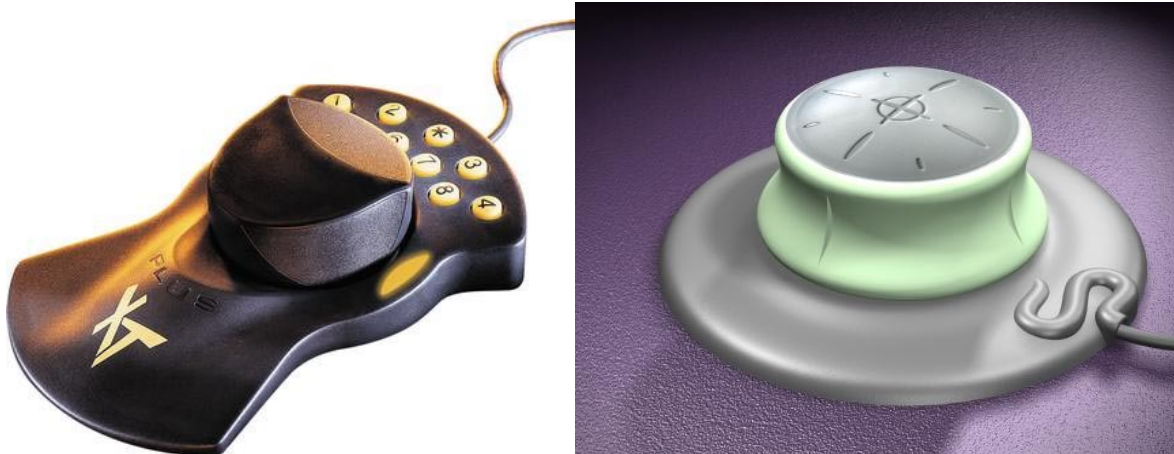
Figure 26: a) Magellan/SPACE MOUSE "Plus XT" (188 x 120 x 44 mm and 720 grams) and b) Cyberpuck (140 x 140 x 45 mm and 510 grams).
