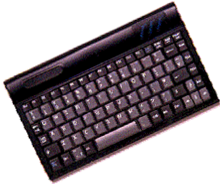
Figure 34: Electrone Model 9001 (10.25 inches wide, about 60% of a standard keyboard).
