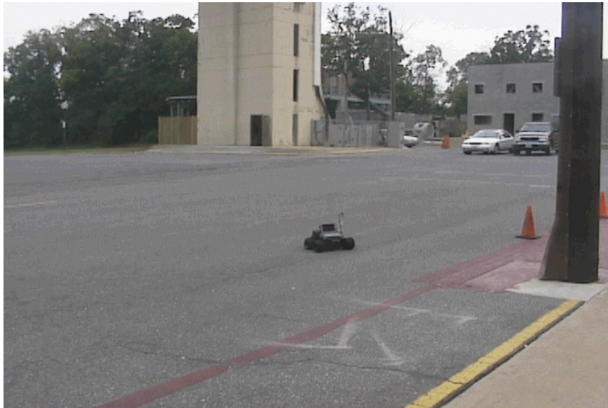
Figure 13: Outdoor approach mission, showing Pioneer AT navigating waypoints toward tower.
