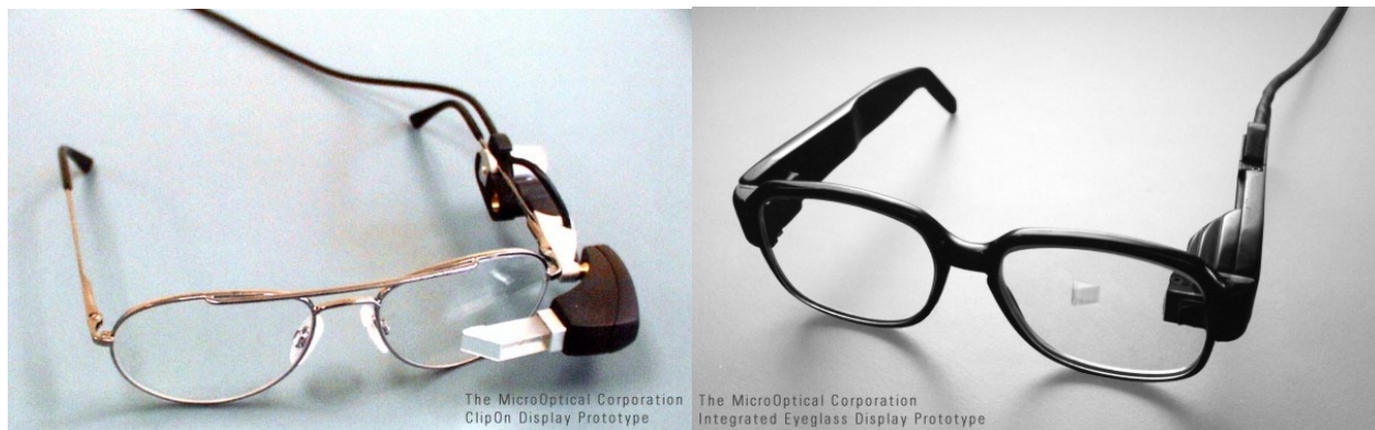
Figure 41: MicroOptical C-1 Clip-On display (a) and integrated eyeglasses (b).
