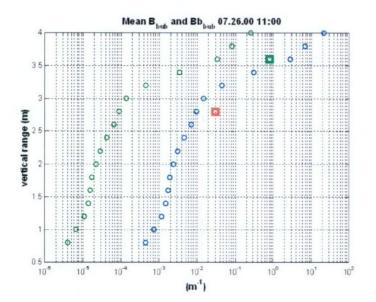
Figure 2. The depth dependence of the light scattering properties of the water due to bubbles. The profile shown was obtained using range gated acoustic techniques (circles) and is representative of the data shown in figure 1. The two squares are values measured by optical instruments and are consistent with the values based upon the acoustic data.
