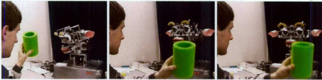
Figure 7: These images are from a sequence in which the instructor wanted the robot to attend to the green object as it moved away from a central location. In the first image the robot is clearly attending; in the second it just as clearly has become fixated on the instructors face. Knowing this prompted the instructor to wave the object a little until it regained the robot's attention.
