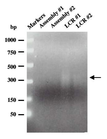
**Figure 26.** Agarose gel of amplified Stx2 B ligase chain reaction (LCR) product. LCR #1 and LCR #2 show LCR bands (~360 bp) amplified from the LCR product first synthesized in figure 25.
