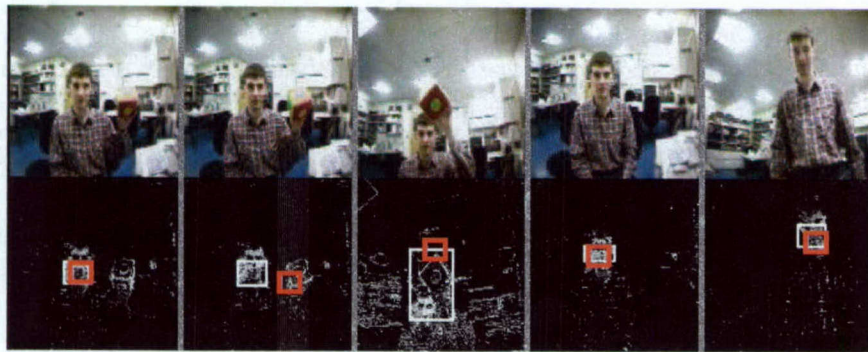
Figure 8-7: Manipulating low-level attention. Images on the top row come directly from the robot's camera. Images on the bottom summarize the contemporaneous state of the robot's attention system. Brightness in the lower image corresponds to saliency; rectangles correspond to regions of interest. The thickest rectangles correspond to the robot's locus of attention. In the first pair of images, the robot (Kismet) is attending to a face and engaging in mutual regard. By shaking the colored block, its saliency increases enough to cause a switch in the robot's attention. The third pair of images shows that the head tracks the toy as it moves, giving feedback to the human as to the robot's locus of attention. The eyes are also continually tracking the target more tightly than the neck does. In the fourth pair of images, the robot's attention switches back to the human's face, which is tracked as it moves.
