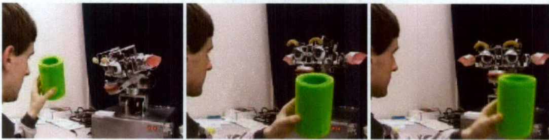
Figure 8-5: These images are from a sequence in which the instructor wanted the robot to attend to the green object as it moved away from a central location. In the first image the robot is clearly attending; in the second it just as clearly has become fixated on the instructors face. Knowing this prompted the instructor to wave the object a little until it regained the robot's attention.
