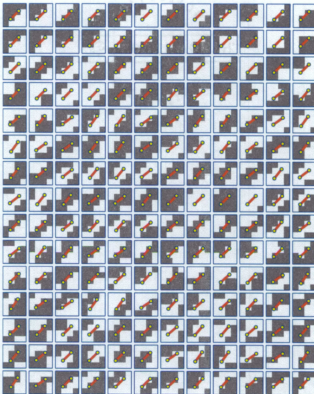
Figure 4-8: The most frequently observed appearances whose orientation is in the range 40 - 50^\circ . Again, there is a clear orientation assigned to many patches that deviate a great deal from "ideal" edges/lines.
