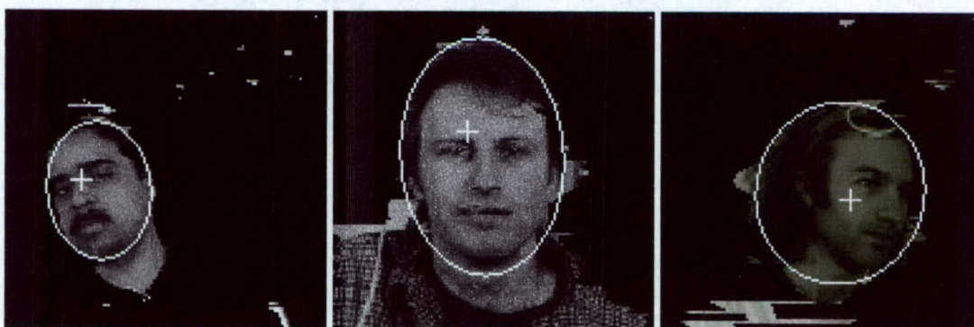
Figure 8-15: Snapshots of the head tracker in action. Hair is problematic. Sometimes it will be included, sometimes not. In individuals with a great deal of hair (rightmost figure), the ellipse can deviate a great deal from the basic shape of the head itself.
