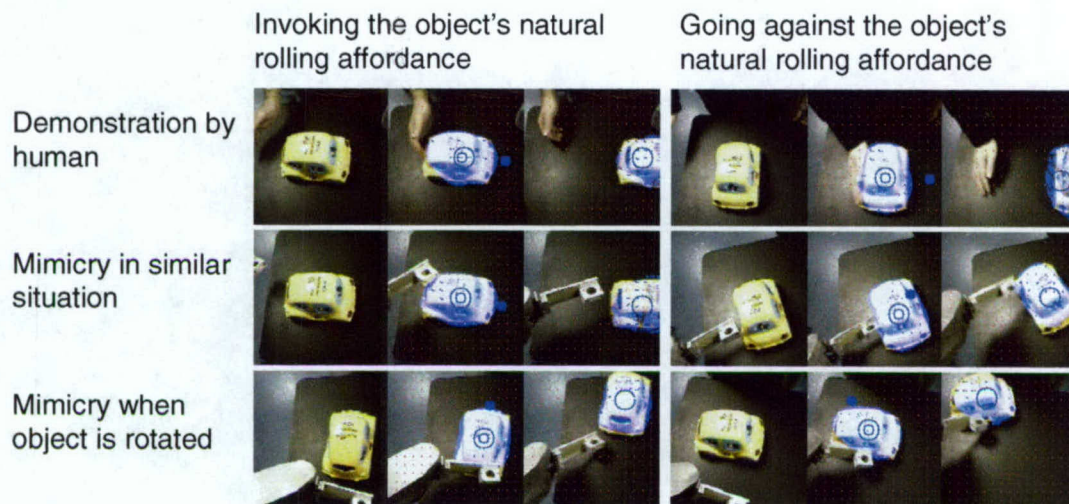
Figure 7-5: A mimicry example using the toy car. The first row shows human demonstration of poking operations, which the robot then mimics. The sequences on the left show the robot mimicking a human exploiting the car's rolling affordance. The sequences on the right show what happens when the human hits the car in a contrary fashion, going against its preferred direction of motion. The robot mimics this "unnatural" action, suppressing its usual behavior of trying to evoke rolling. Mimicry is shown to be independent of the orientation at which the car is presented.
