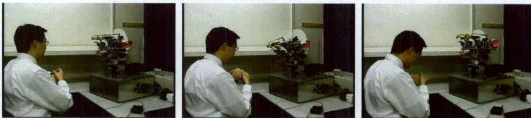
Figure 8-6: Kismet interacting with a test subject unacquainted with the details of the robot's implementation and behavior. The subject decides to show Kismet his watch, so he brings it forward and taps it (left). Motion plus size plus skin-color makes this an attractive target and Kismet looks at it (center). Once the motion stops, Kismet looks away (right).
