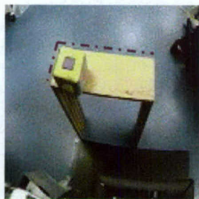
Figure 2: A cube on a table. The edges of the table and cube happen to be aligned (dashed line), the colors of the cube and table are not well separated, and the cube has a potentially confusing surface pattern.
