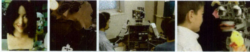
Figure 1. A sampling of robots designed to interact with people. The far left picture shows a realistic face robot designed at the Science University of Tokyo. The middle left picture shows WE-3RII , an expressive face robot developed at Waseda University. The middle right picture shows Robita , an upper-torso robot also developed at Waseda University to track speaking turns. The far right picture shows our expressive robot, Kismet , developed at MIT. The two leftmost photos are courtesy of Peter Menzel [8].
