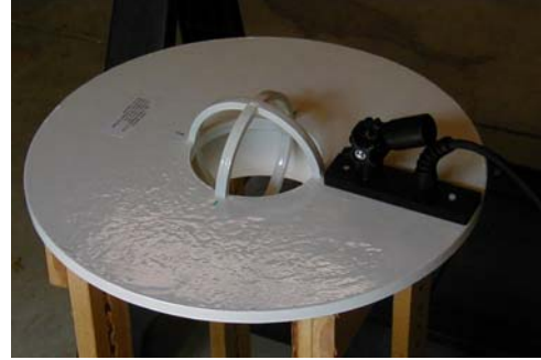
Figure II-13. Three Receiver Coils on the EMI Sensor Head Measure Three Vector Components of Target Response Over Ultra-Wideband.
