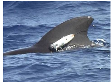
Figure II-4. The Digital Acoustic Recording Tag Developed by Woods Hole Oceanographic Institute.
