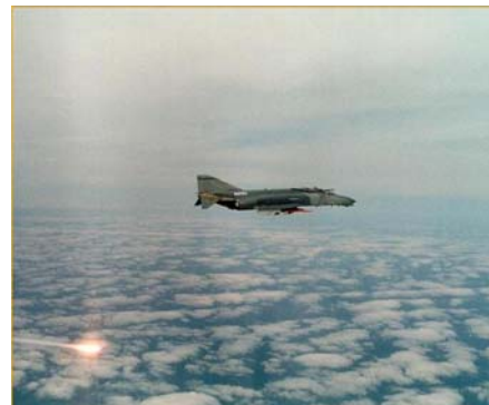
Figure II-2. Infrared Decoy Flare Being Deployed from an F-4 Phantom.
