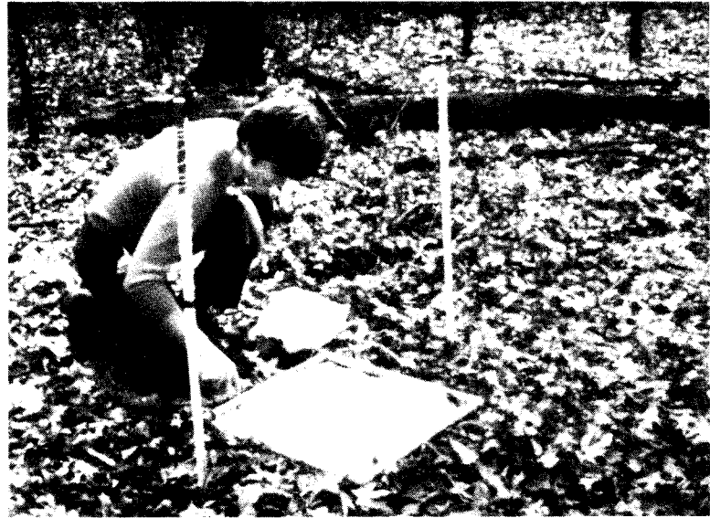
Figure 3. Researcher spreading a feldspar clay pad for a marker horizon
