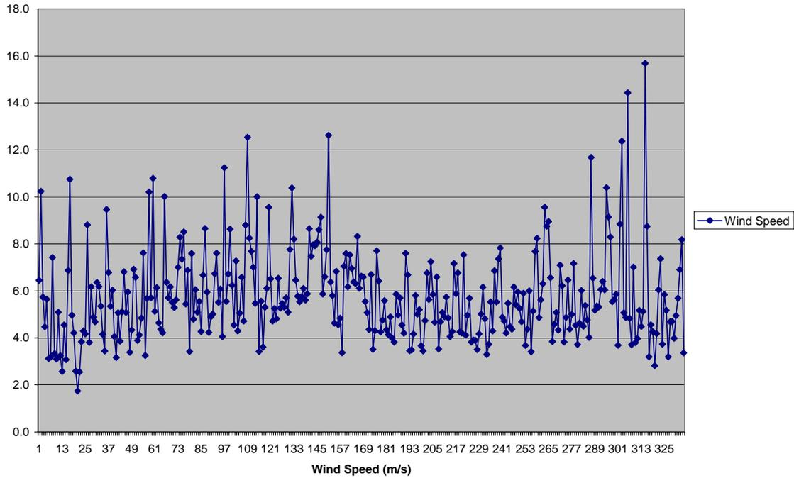
The average daily wind speed at Peterson AFB is at or above the cut-in speed of 4  $\text{ms}^{-1}$  85% of the time for the 1.5 MW, 62 m NEG Micon turbines.
