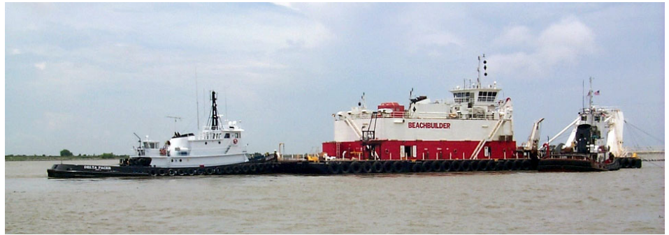
Figure 4. Stern tug used to maneuver Beachbuilder
