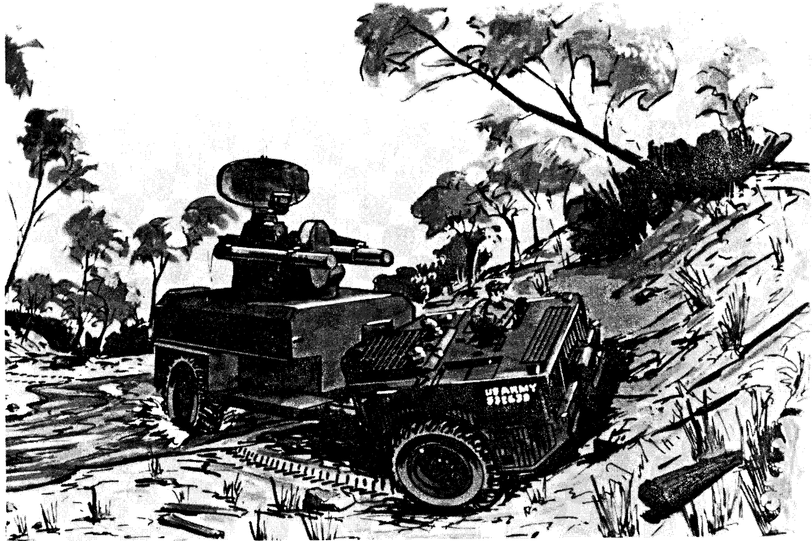
Artist's Conception of the SHORAD (ROLAND II) System Mounted on the GOER Vehicle - 43,000 lbs.
