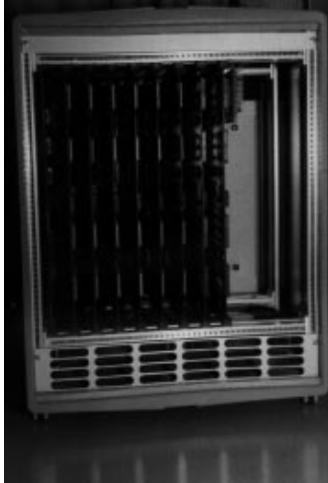
Figure 3: MIT Laboratory for Computer Science cellular automata machine CAM-8. This 8 module prototype can evolve a D-dimensional cellular space with 32 million sites where each site has 16 bits of data with a site update rate of 200 million per second. The communication network is a Cartesian three-dimensional mesh. Crystallographic lattice geometries can be directly embedded into the CAM-8.
