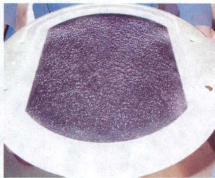
Figure 3B Large Area Carbon Microfiber Array
