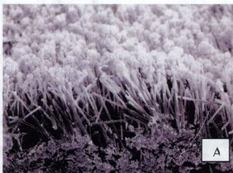
Figure 3A. Cross Section of CPS Catalyzed Carbon Microfiber Electrode
