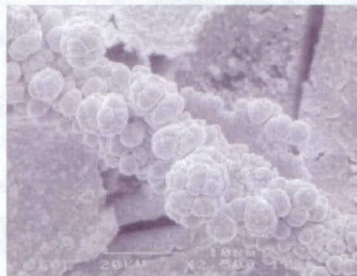
Figure 3C Pd:Ir Nodules on Carbon Paper
