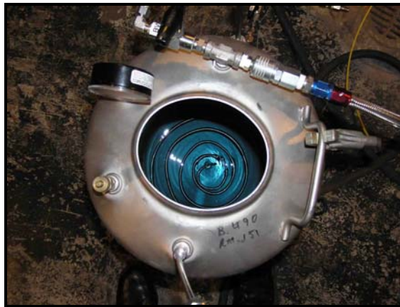
Figure 18. Top view of fuel conditioning holding tank with nitrogen bubbling coiled tube at the tank bottom
