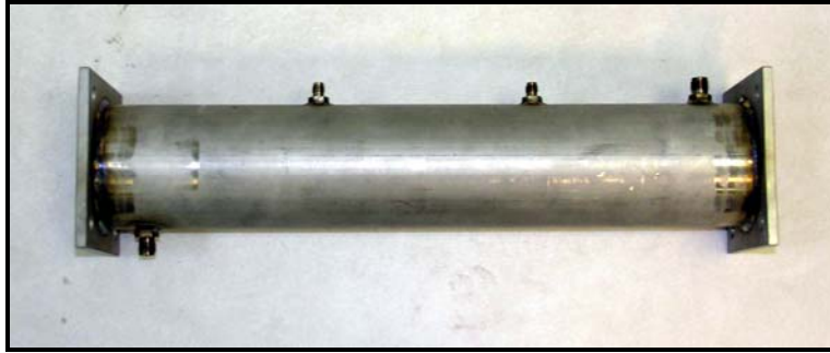
Figure 23. Profile view of short heat exchanger with inlet and outlet ports at opposing ends and two spaced thermocouple flow ports on the outlet side
