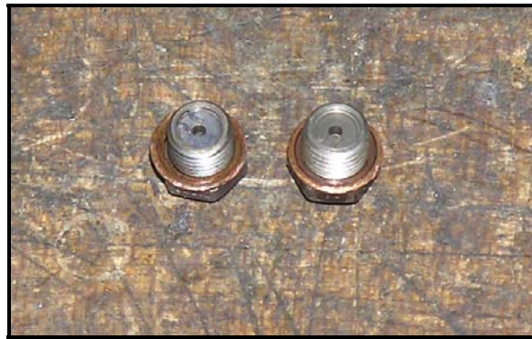
Figure 58. JP-8 fuel nozzles pretest condition
