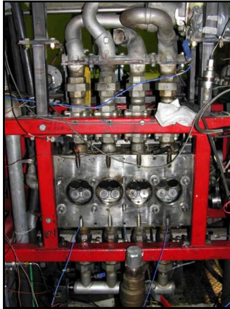
Figure 19. GM Quad 4 head being used as PDE valve train for fill air manifold (top) and purge manifold (bottom)
