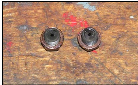
Figure 59. JP-8 fuel nozzles posttest condition
