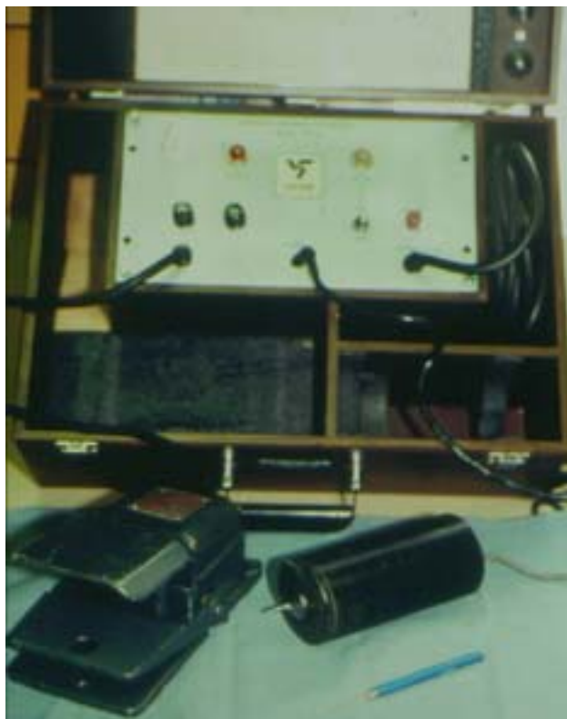
Fig. 14-8. The Bronson electromagnet, consisting of the amplifier box, foot pedal, and a large, handheld magnet.
