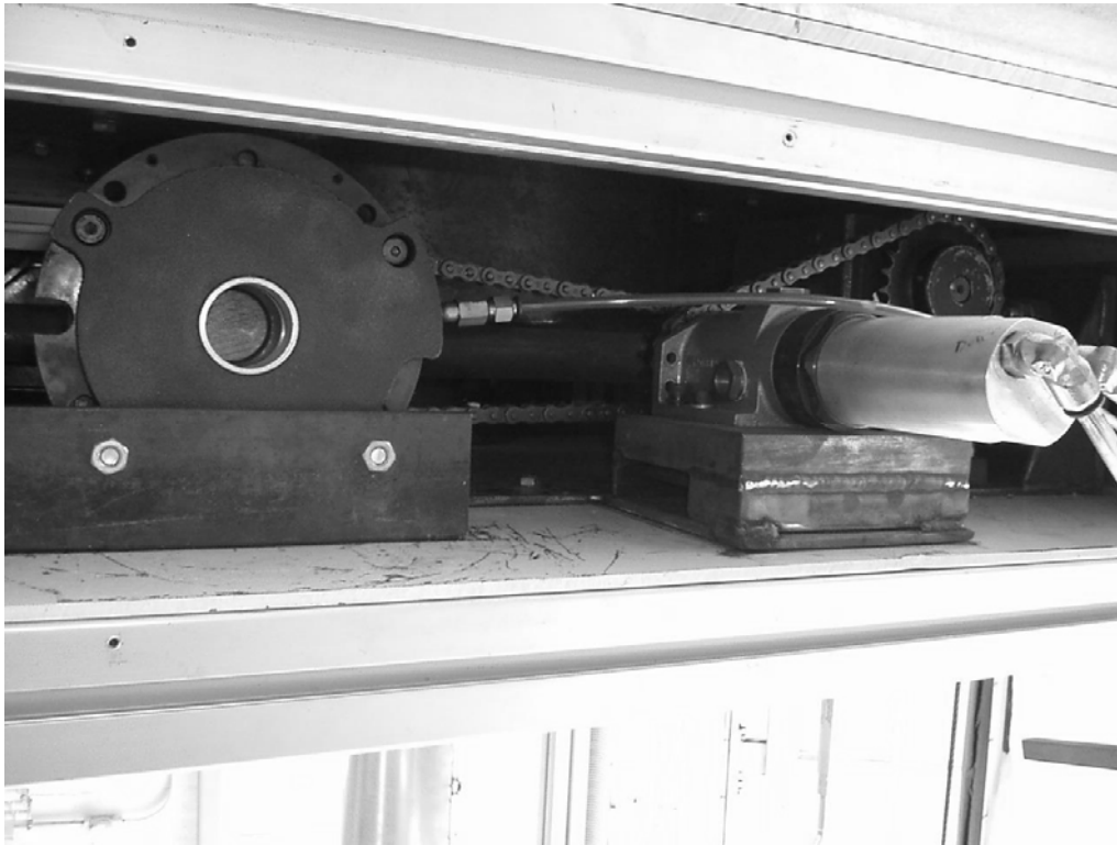
Figure 33. Chain drive for cab lift power transmission.
