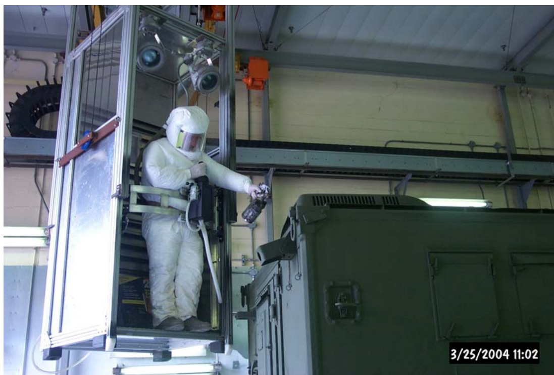
Figure 36. Painter in modified Mobile Zone cab.
