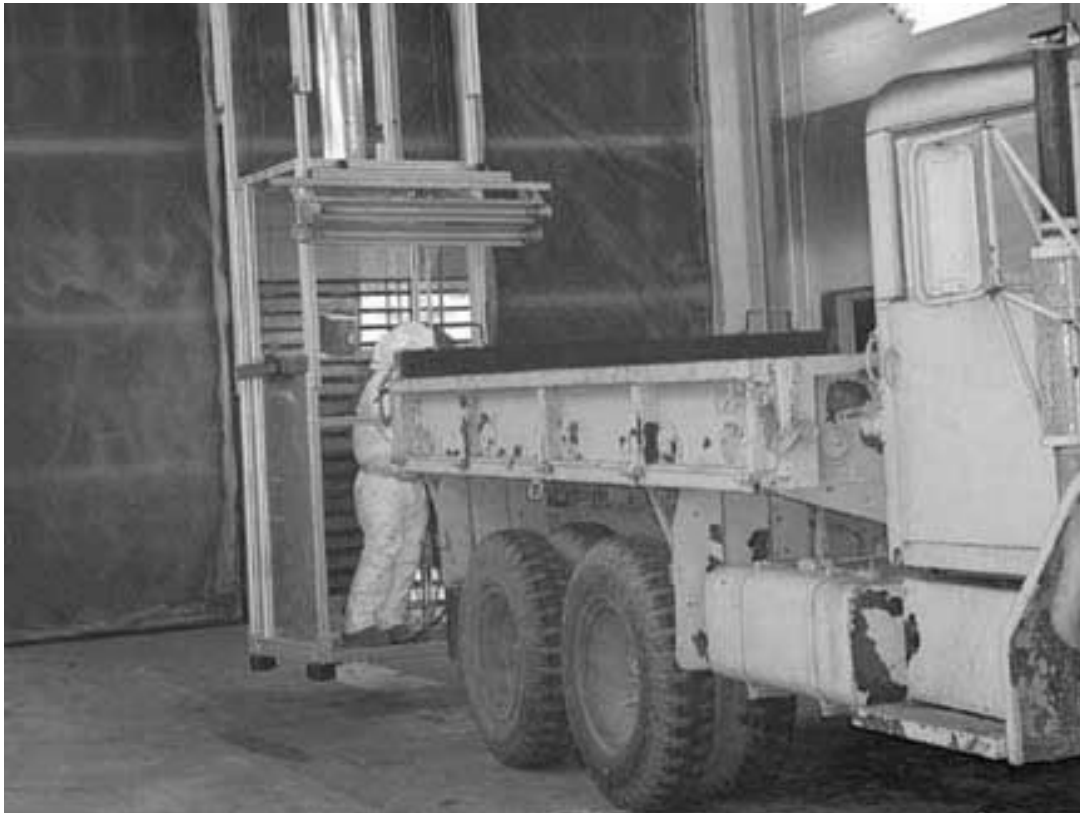
Figure 28. Painting the back end of a truck using the Mobile Zone cab.
