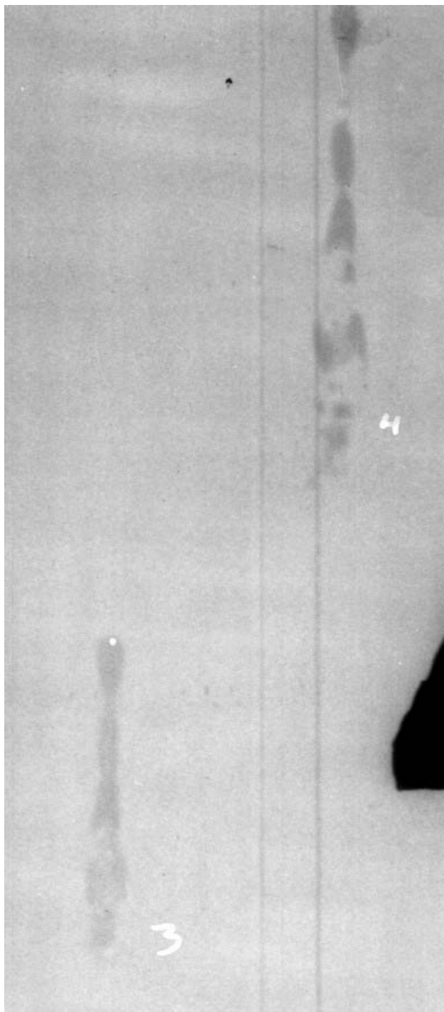
Figure 9. RP-4 SFF EBW shot No. 778. (X-ray flash times are 50.6 and 75.5 \mu s.)
