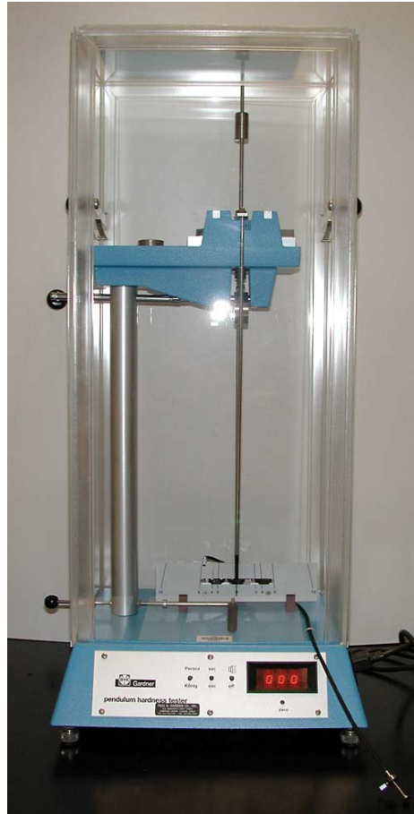
Figure 13. König pendulum damping coating hardness test apparatus (ASTM D 4366).
