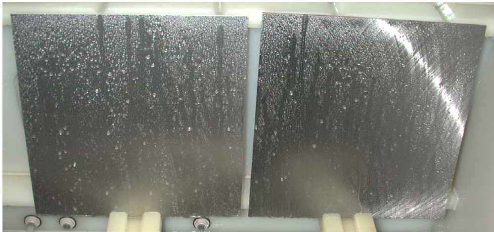
Figure 52. Initial appearance of wet 2-day ambient dwell CorrosionX Aviation-treated plates: aluminum (left) and steel (right).
