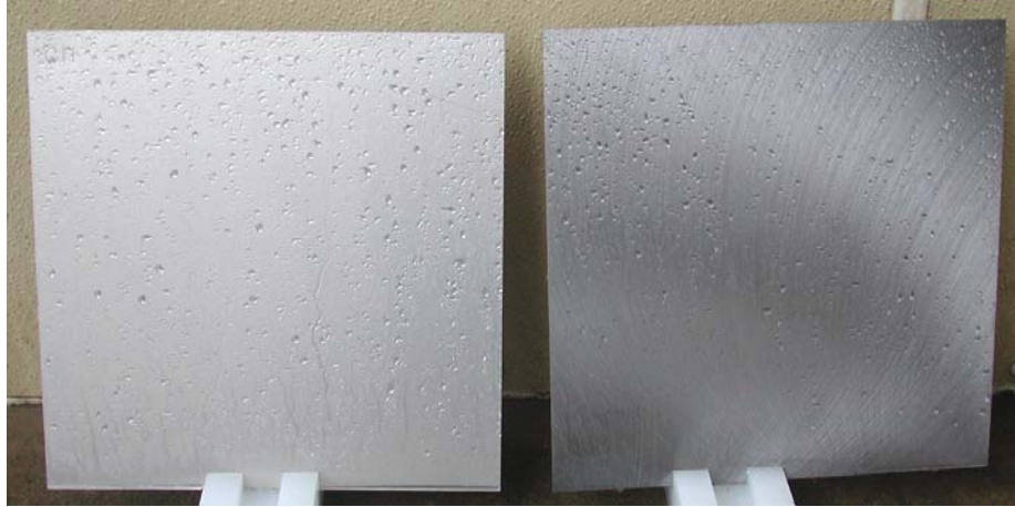
Figure 62. Appearance of wet 2-day 60 °C baked Carwell AR500-treated plates after two pressure washes: aluminum (left) and steel (right).
