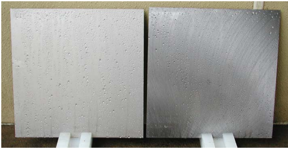
Figure 63. Appearance of wet 2-day 60 °C baked Carwell AR500-treated plates after three pressure washes: aluminum (left) and steel (right).
