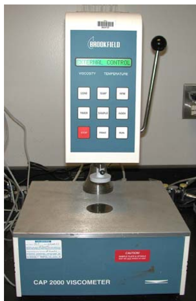
Figure 12. Cone/plate viscometer (ASTM D 4287).
