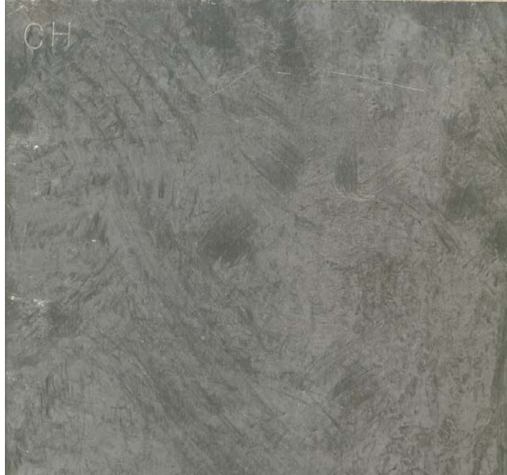
Figure 65. Appearance of residual film on dry 2-day 60 °C baked Carwell AR500-treated plates after four pressure washes on aluminum.
