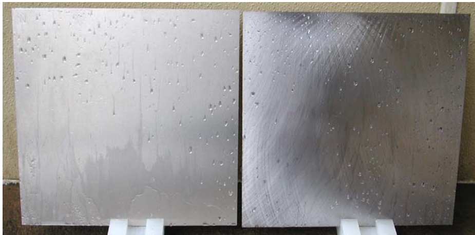
Figure 55. Appearance of wet untreated plates after one pressure wash: aluminum (left) and steel (right).
