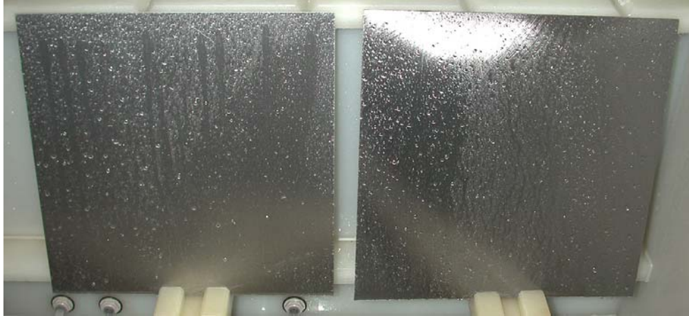
Figure 51. Initial appearance of wet 2-day ambient dwell Carwell AR500-treated plates: aluminum (left) and steel (right).
