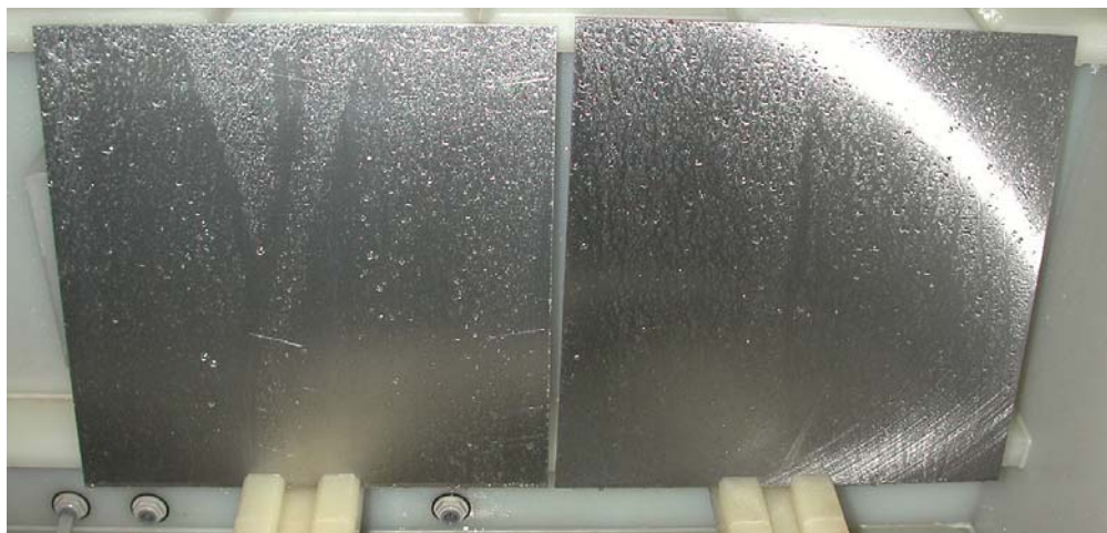
Figure 53. Initial appearance of wet 2-day 60 °C baked Carwell AR500-treated plates: aluminum (left) and steel (right).
