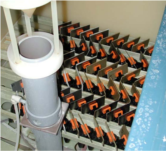
Figure 10. Crevice corrosion sandwich specimen chamber layout.
