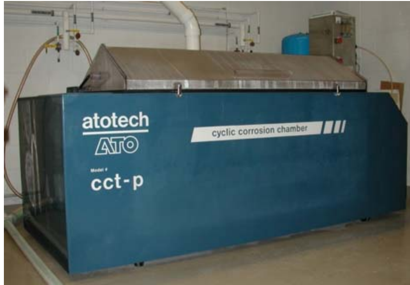
Figure 1. Test chamber configuration used for GM 9540P cyclic corrosion.
