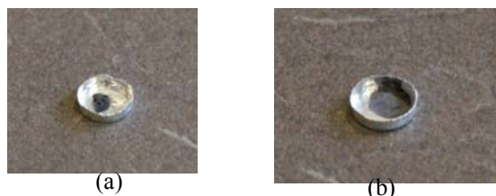
Figure 9. Comparison of TGA residues of electrospun fibers: (a) 5050-MMT, (b) 5050-FH.
