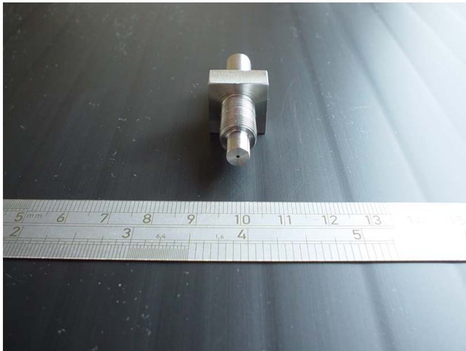
Figure 2. Typical Catalyst Injector (0.7 mm Orifice)
