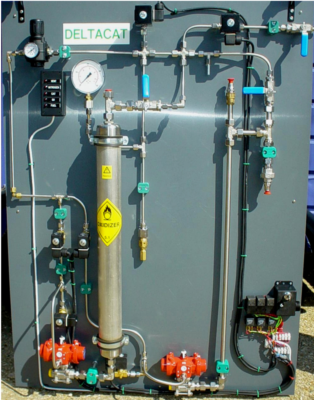
Figure 6. Propellant Delivery System
