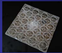
PMMA discs uniformly distributed in PC
