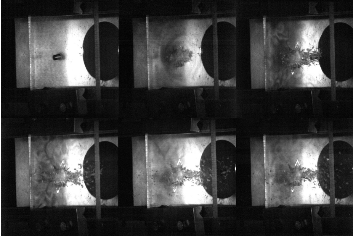
Figure 7. High-speed photographs of impact on 9.25 mm PMMA plate at 430 m/s (each frame is 25 \mu s apart)
