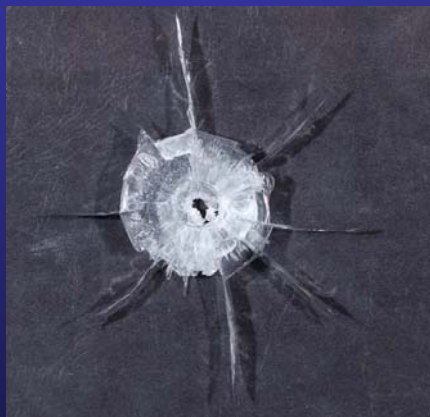
Catastrophic cracks in PMMA
