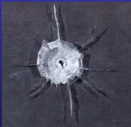
Catastrophic cracks in PMMA
