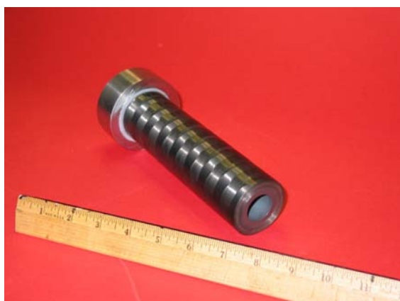
Figure 3 - Overwrapped ceramic tube for ballistic testing.
