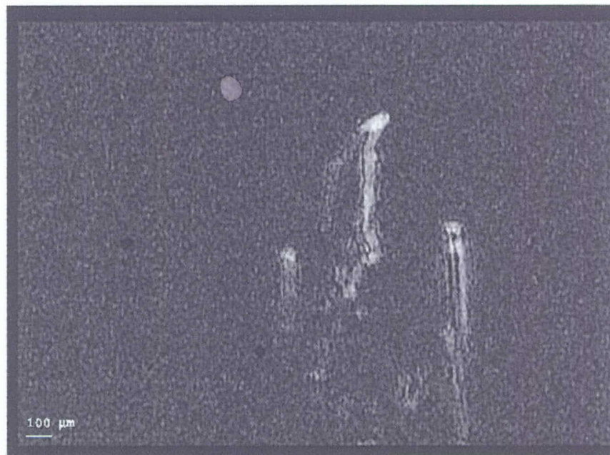
Figure 4.6 1-Propanol Droplet at x = 0.3089 in (7.85 mm) S = 3.6755 , Model v_r = 1447 ft/s (441 m/s), Model M_r = 2.594 , Model We = 616 , Model Re = 1811
