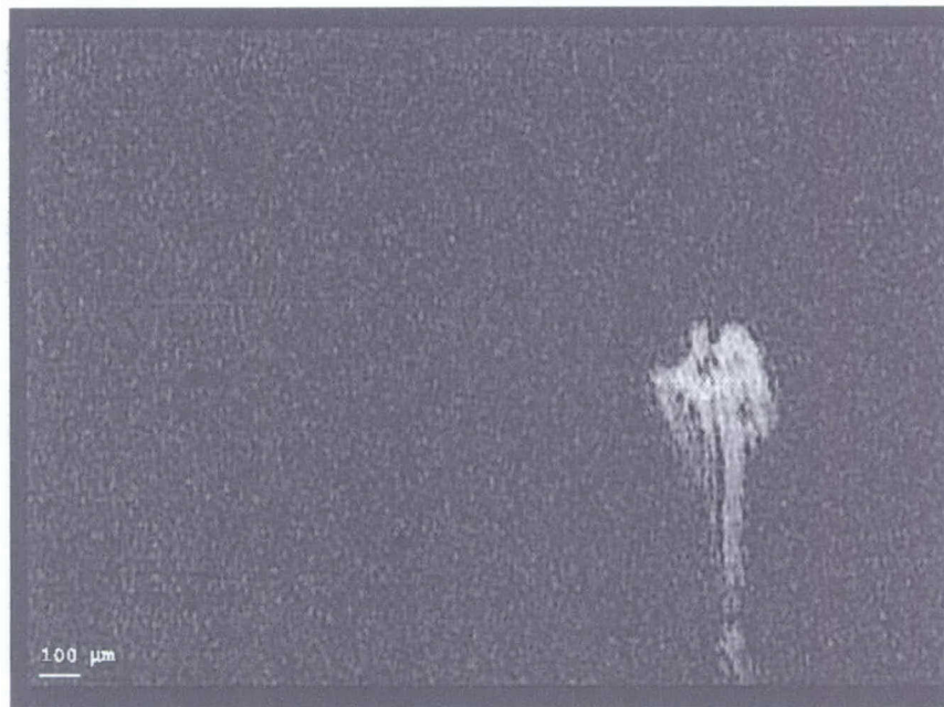
Figure 4.5 1-Propanol Droplet at x = 0.2622 in (6.66 mm) S = 2.2172 , Model v_r = 1459 ft/s (445 m/s), Model M_r = 2.434 , Model We = 626 , Model Re = 1827
