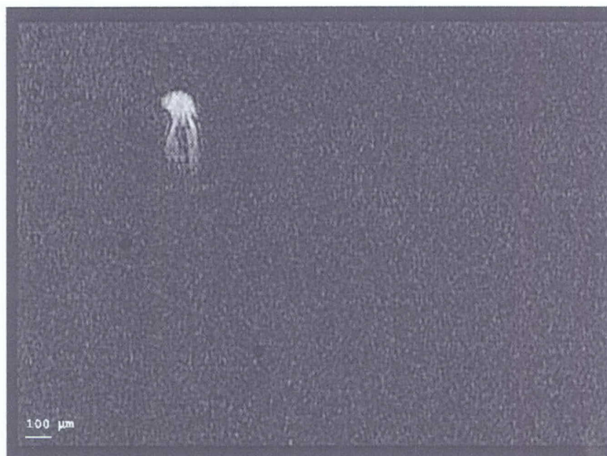
Figure 4.11 Ethanol Droplet at x = 0.0692 in (1.76 mm) S = 0.1965 , Model v_r = 1207 ft/s (368 m/s), Model M_r = 1.272 , Model We = 429 , Model Re = 1512
