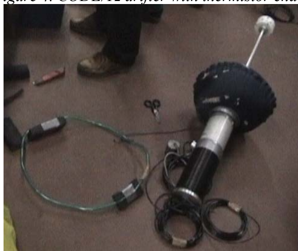
Figure 5. CMOD (XAN-3) drifter with thermistor chain.
