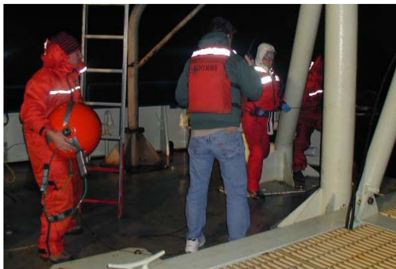
Figure 6. Deploying an optical drifter (SVP/OCM) from the stern.
