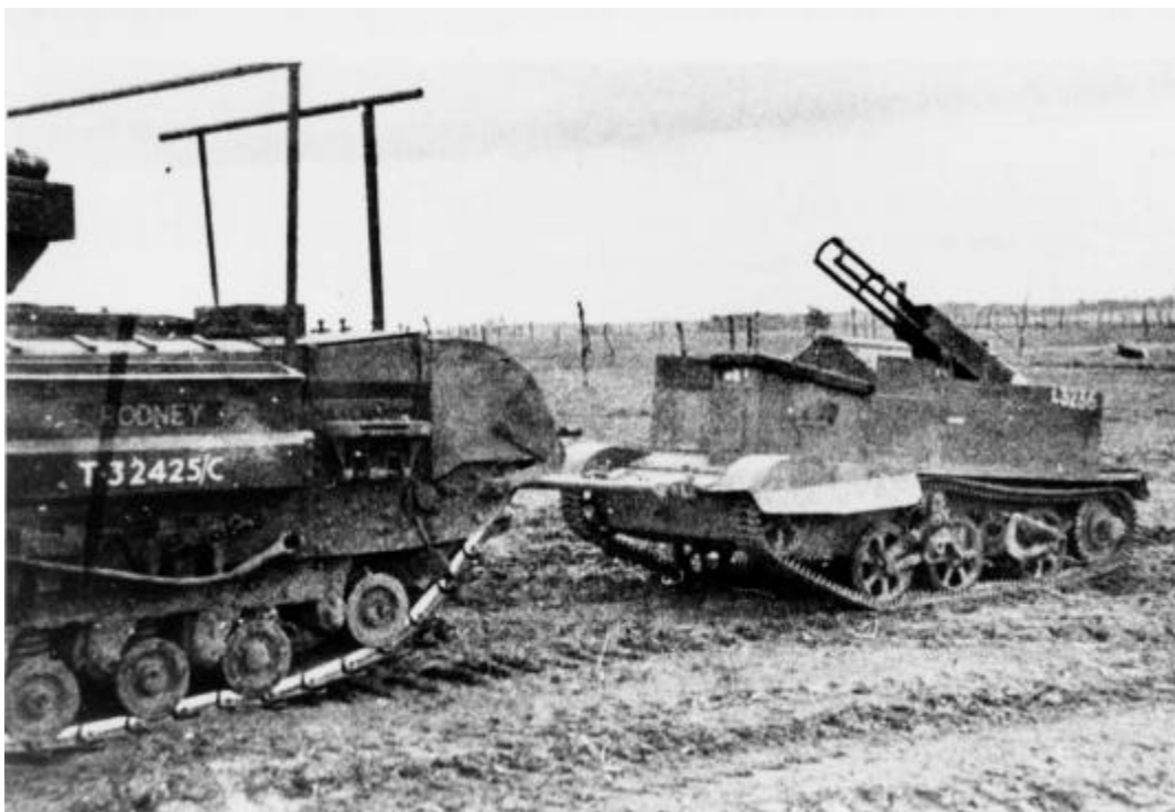
Fig. 5. AVRE towing Conger explosive rocket. Reprinted with permission of The Tank Museum, Bovington, Dorset, England.
