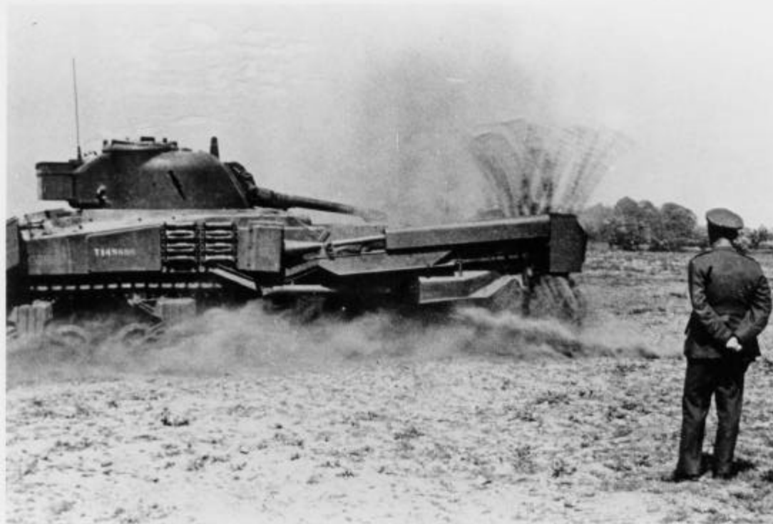
Fig. 6. Sherman Crab in operation, with observer dangerously close to the action. Reprinted with permission of The Tank Museum, Bovington, Dorset, England.
