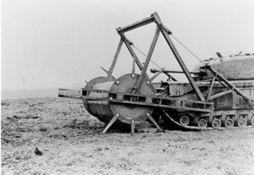
Fig. 4. Churchill with “Bobbin” device. Reprinted with permission of The Tank Museum, Bovington, Dorset, England.
