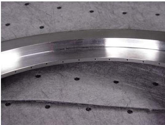
**Figure 4: Inconel Jet Ring Containing 48 Fuel-Air Jets.**
