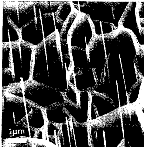
Fig. 6.4. Metal nanowires and nanowalls grown at 925°C in a process utilizing gold surface diffusion and aggregation at nodes. (Courtesy Dr. M. Meyyappan, NASA/Ames Research Center)
