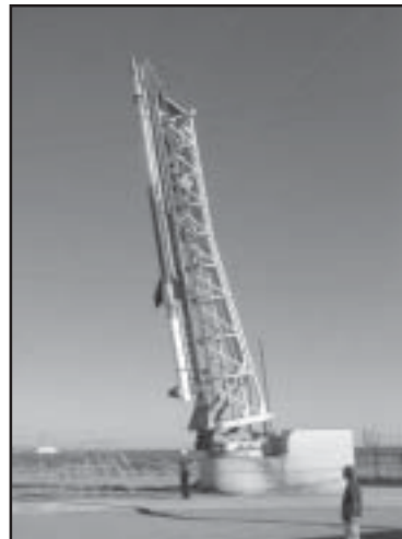
A Black Brand rocket being readied for flight at the White Sands Missile Range. The rocket is carrying NRL's advanced spectrometer for studying stars at soft X-ray wavelengths.
