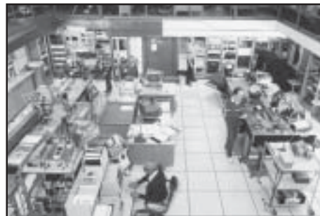
The Missile Seeker Evaluation Facility is a computerized facility that is used to evaluate optical countermeasures to infrared missile seekers and infrared imaging sensors
