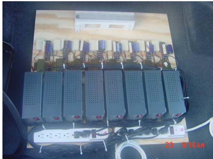
Figure 3.13 – 8 Loop GITI Analog Controls Wired on Board
